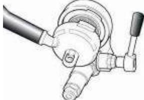
A line drawing showing the filter holder being clamped into the brew group.                                   |
