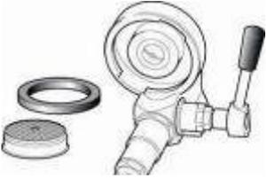
A line drawing showing the new shower screen and group gasket ready for installation, with the rounded side of the gasket facing upwards. | <p>6<br/>Clean the brew group with a brush.<br/>Lock the shower screen firmly into the gasket.</p>
